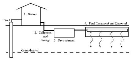
Components of an onsite wastewater treatment system.
